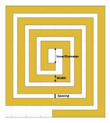
Consider a square spiral inductor from "Inductors and Capacitors". Calculate and plot the S-parameters to show the power conservation at the default frequency of 600 MHz.
