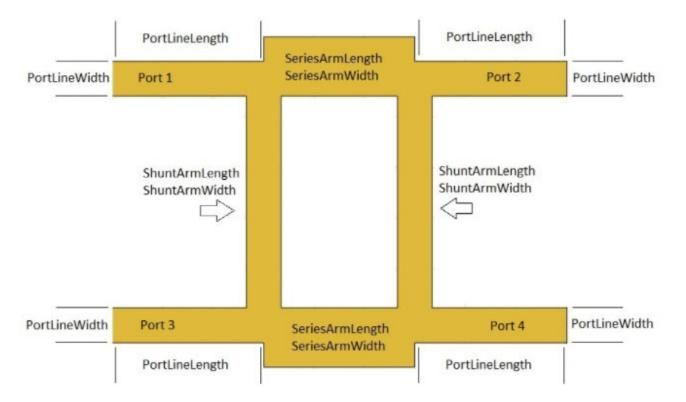
Consider the branchline coupler from "Splitters and Couplers". The parameter values of this coupler are for a design frequency of 3 GHz. Calculate and plot the S-parameters of this coupler to understand its behavior.
