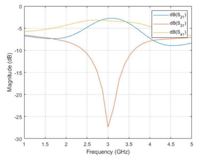
The transmission coefficients of  $S_{21}$  and  $S_{41}$  show that the power is equally divided between Port 2 and Port 4.  $S_{31}$  is -30 dB as Port 3 is isolated.
