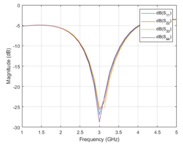
All the reflection coefficients  $S_{11}$ ,  $S_{22}$ ,  $S_{33}$ , and  $S_{44}$  are close to -30 dB showing that the default branchline coupler has a good match at all ports.
